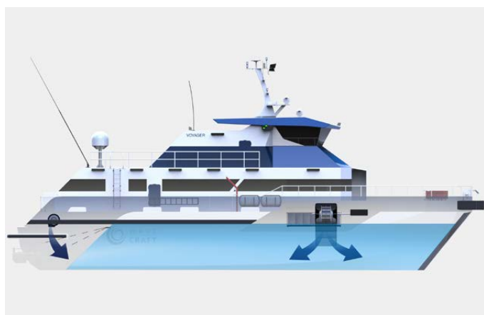
Surface-effect ship (SES) technology
